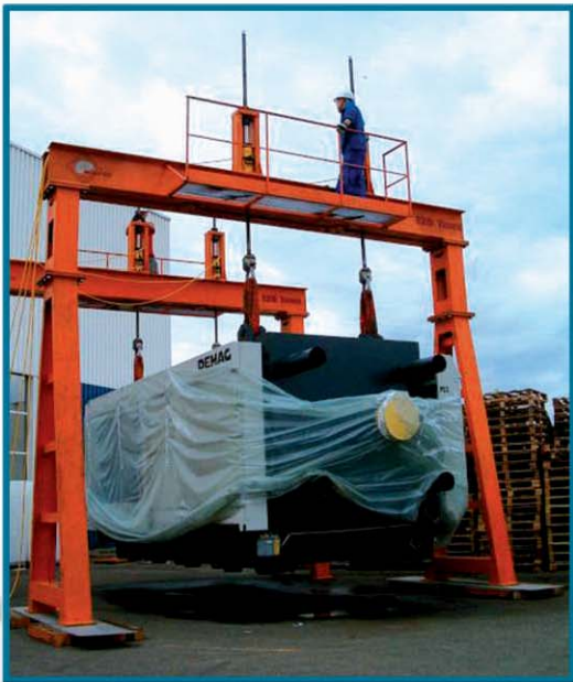
Loading of a pressing element of DEMAG machine – 60 tonnes.
